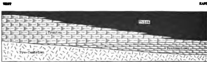
FIG. 1110. — Diagrammatic east-west section showing the replacing relationships of the "Utica" shale and Trenton limestone (replacing overlap). Note that the age of the basal black shale members differs in the different regions and that there is conformity throughout.
